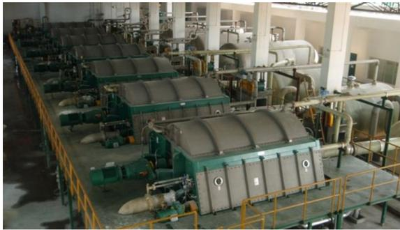
Together with GL&V, Microfusion assisted in the implementation of the GL&V DualC™ cooking process at the Chongqing mill. The DualC™ cooking process combines two-stage black liquor impregnation with a carefully controlled alkali and temperature profile specifically derived for bamboo cooking for optimal issue strength and properties. The cooking and washing process is completely automated and optimized using ABB 800xA DCS.
